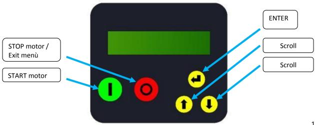
Screen is a back-light LCD displaying 2 rows of 16 digits each. If the menu indication is longer than 16 digit, the row will scroll-
