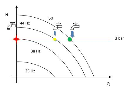
Progressively closing the delivery valve water reduces flow causing VASCO to reduce the pump speed by reducing the output frequency, to maintain constant the pressure (i.e. 3 bar).
