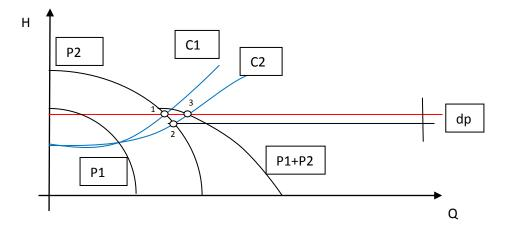
If pump 1 (P1) is already running to grant the desired set pressure (red line), an additional water request change the system curve from C1 to C2; being P1 at maximum speed, it is not possible to maintain the set pressure by increasing the speed so the system pressure will drop till reaching the new working point 2.
